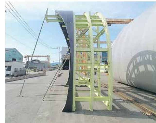
擦り付け型枠
